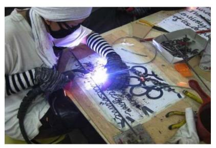
Figure 3: Production of wall installations by electro welding (Source: Mr. Tang Mun Kian (2016).)
